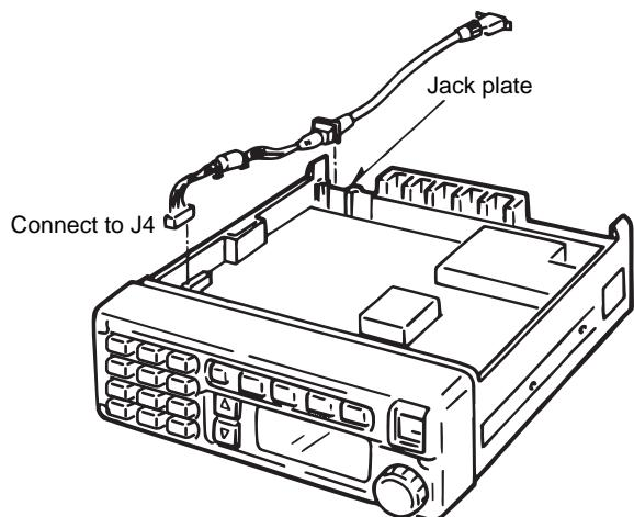
Break the jack plate using cutting pliers to connect the OPC-617.
