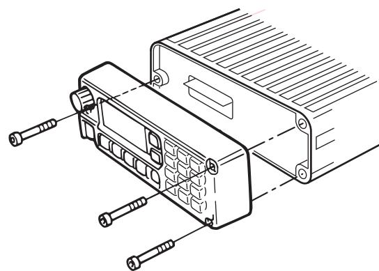
③ Attach the 'RMK-1 rear unit attachment' to the transceiver main unit using the supplied screws.
