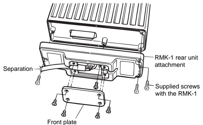
⑦ Remove 4 screws from the 'RMK-1 front unit attachment' to open the rear plate.
