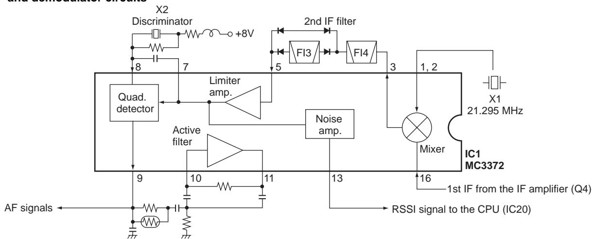
through the matching circuit (L15, L52) and a pair of crystal filters (FI1) in order to obtain selection capability and to pass only the desired signals. The filtered signal is applied to the 2nd IF circuit after being amplified at the 1st IF amplifier (Q4).
